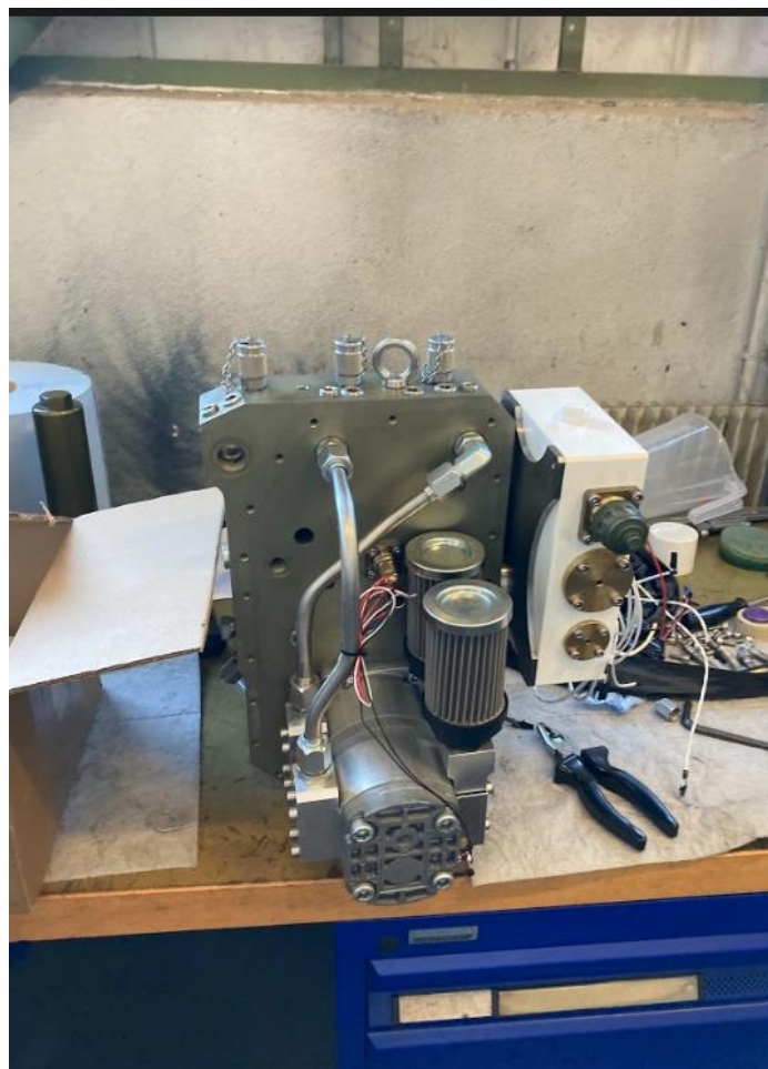
The hydraulic central of ROV Victor 6000 we put in hyperbaric chamber and on which I had to add a thermal exchanger.
